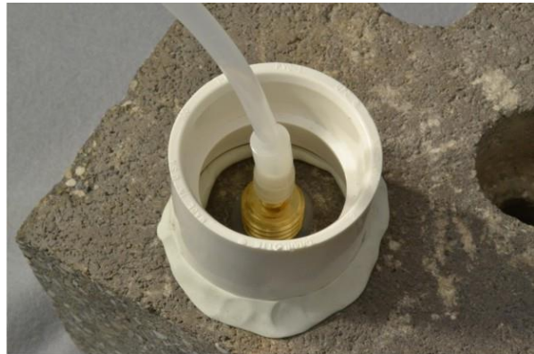
Figure 8. Water dam used for leak detection
